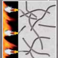
With PP fibers Fibers are melting, channels are made, steam can escape.
